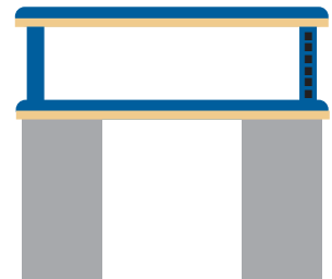
PART NO. INCLUDES TB0602- (2) 16" instrument riser supports (1 with power) 12" deep instru. riser shelf worksta. + shelf back stops
