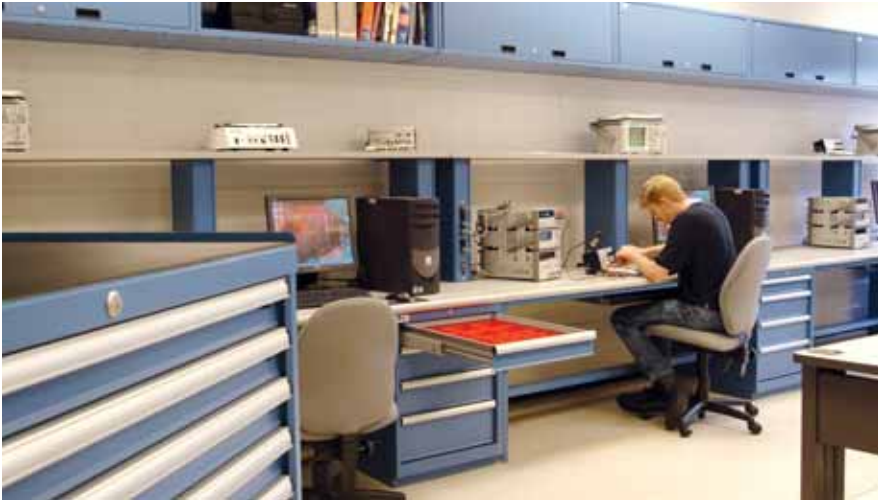
Technical electronic workstations can be outfitted with cabinet pedestals for easy access to stored tools and parts.
